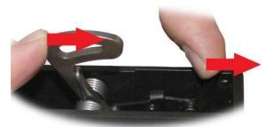
5) To reinstall your trigger housing assembly you'll need to make sure the hammer is engaged with the sear. To do this, you might need to simultaneously pull back on the trigger linkage bar if it fell down during installation. Follow your owner's manual to reassemble your rifle.
